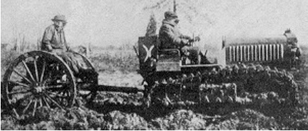
Experience in World War I alerts the Army to the difficulties in moving their newer, but heavier artillery pieces on the battlefield. Using commercial tractors seems like a quick solution to the problem. Exhaustive tests begin on automotive equipment. Tractor shown is the model 1922 Aberdeen
